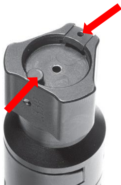
FIGURE 88 Apply one drop of lubrication on the ex- tractor and one drop on the ejector.
